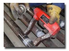
Ultrasonic on most materials and welds
